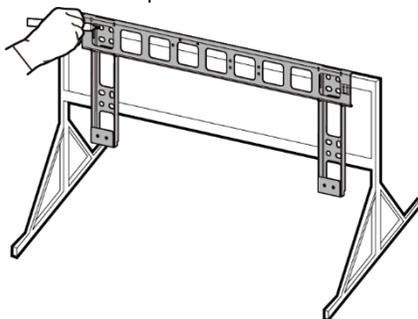
3. Drill holes. (You are advised to apply anti-rust paint on the hole positions for protection.)
